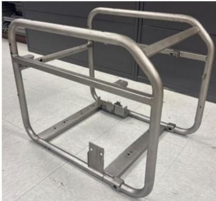
Figure 9: Painted Generator Chassis
