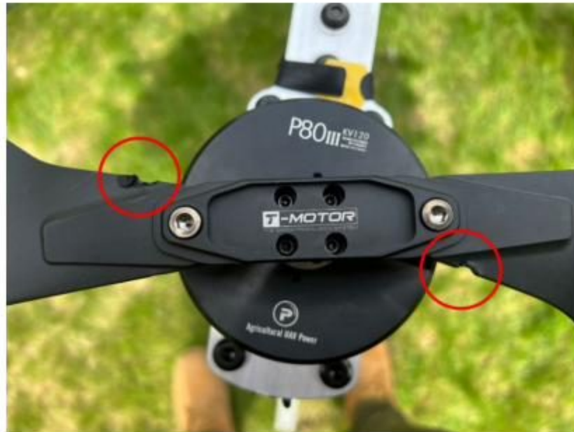
Figure 4943: Blade Damage Caused by Acceleration
